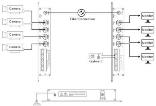
To install, connect the video inputs to the SWV60401-T, connect the video monitors or other video receptors to the SWV60401-R, and connect an appropriate optical fiber between the SWV60401-T and SWV60401-R optical ports. Connect data signal sources or destinations, as required, to the "DATA" port per the following Built-In Data Connection section.
