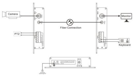
To install, connect the video inputs to the SWV60101-T, connect the video monitors or other video receptors to the SWV60101-R, and connect an appropriate optical fiber between the SWV60101-T and SWV60101-R optical ports. Connect data signal sources or destinations, as required, to the "DATA" port per the following Built-In Data Connection section.
